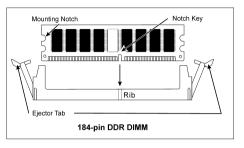
both sides of the slot automatically snaps into the mounting notch. Do not force the DIMM module in with extra force as the DIMM module only fit in one direction.
