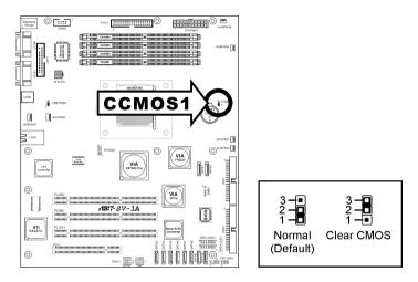
**WARNING:** Turn the power off first (including the +5V standby power) before clearing the CMOS memory. Failing to do so may cause your system to work abnormally or malfunction.
