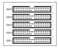
These four ports are controlled by HighPoint HPT374 chipset that supports regular Ultra ATA/133 devices ports or a RAID array in the combination of RAID 0, RAID 1, or RAID 0+1 mode. Each port connects up to two drives.
