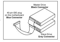
**NOTE:** The red line on the ribbon cable should be aligned with pin-1 on this connector.
