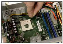
Locate the CPU socket on the motherboard. Pull the CPU socket lever sideways away from the socket and then upwards to vertical position.
