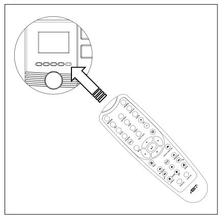
This remote controller is powered by two AAA-size batteries. Point the infrared transmitter of the remote controller to the infrared receiver sensor on the front panel when accessing a remote command.
