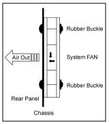
Identify the air-blow direction. Make sure to install the fan so as to blow the air out.
