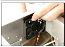
Fasten the system fan to the chassis with four rubber buckles.
