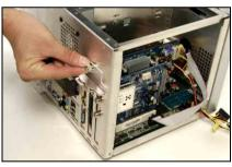
Screw back the I/O shield support by fingers.
