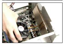
Align the thermal module toward the heat-sinking hole at rear panel.
