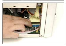
Connect the other side of the IDE cable to the IDE1 connector on motherboard.
