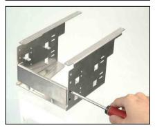
To install a second optical drive, the shielding plate that was originally secured at the lower layer has to be removed first.
