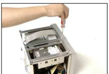
Fasten the hard-drive holder to the chassis.
