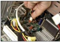
Connect the fan-power plug of the system fan to the AUX FAN1 header on motherboard.
