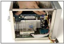
Press down the AGP or PCI add-on card into the slot.
