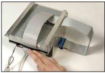
Connect the signal and audio cable to the optical drive.
