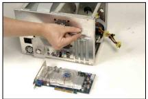
Unscrew the I/O shield support.
