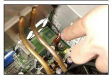
Connect the fan-power plug of the fan-duct to the SYSFAN1 header on motherboard.
