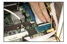
Connect the other side of the optical-drive cable to the IDE2 connector on motherboard.
