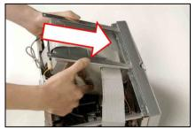
Slide in the holder into the chassis by 45 degree.
