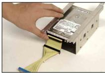
Connect the signal cable to the hard drive.
