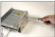
Install one optical drive into the upper layer of drive holder. Fasten the optical drive to the drive holder.
