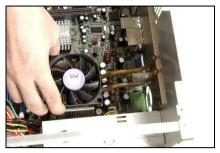
Put the thermal module onto the CPU die. Align the four screws on thermal module with the four screw holes on motherboard.
