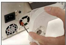
Pass the fan-power plug of the fan-duct through the I/O shield into the chassis.
