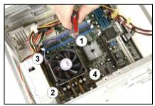
Fasten the four screws on thermal module by the order of 1 through 4.
