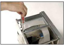
Fasten the optical-drive holder to the chassis.
