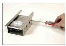
Install one IDE hard drive into the bay. Fasten the hard drive to its holder.
