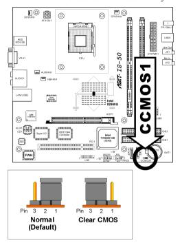
**ATTENTION:** Turn the system power off first (including the +5V standby power) before clearing the CMOS memory. Failing to do so may cause your system to work abnormally or malfunction.
