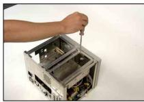
Unscrew the optical-drive and hard-drive holder.
