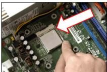
Insert the CPU with the correct orientation. Do not use extra force to insert CPU; it only fits in one orientation. Close down the socket lever while holding down the CPU.
