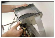
Connect the power cord to optical drive.
