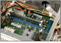
The memory module is firmly installed.
