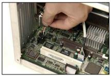
Connect the audio cable from the connector of audio-out on optical-drive to the CD1 on motherboard.
