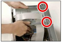
Align the screw holes with the holes on the chassis.
