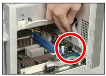
Connect the card-reader plug back to FP-USB1 header.
