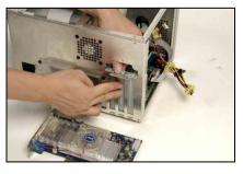
Take off the I/O shield of the slot you want to install add-on card.
