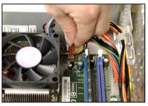
Connect the fan-power plug of the thermal module to the CPU FAN1 header on the motherboard.
