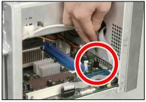
Pull out the card-reader plug from FP-USB1 header.
