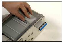
Pass the optical drive cable through the cable hole.
